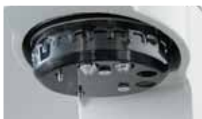
Power turret with 2 indenter mounts and 4 objective mounts (manual operation possible)
