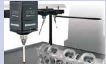
MPP-10 For effective screw depth measurement
