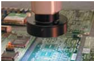
QVP (Quick Vision Probe) For video measurement
